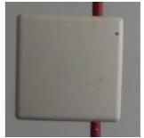
Figura 3.3: Antena 5.5 GHz
